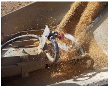
Spraying Activist Zinc onto seed as it travels up the auger
